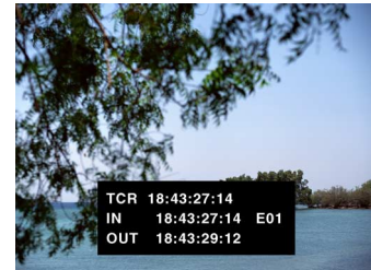
(Event screen) Register or change the IN and OUT points while viewing the images. Set the SUPER switch to ON before proceeding.
